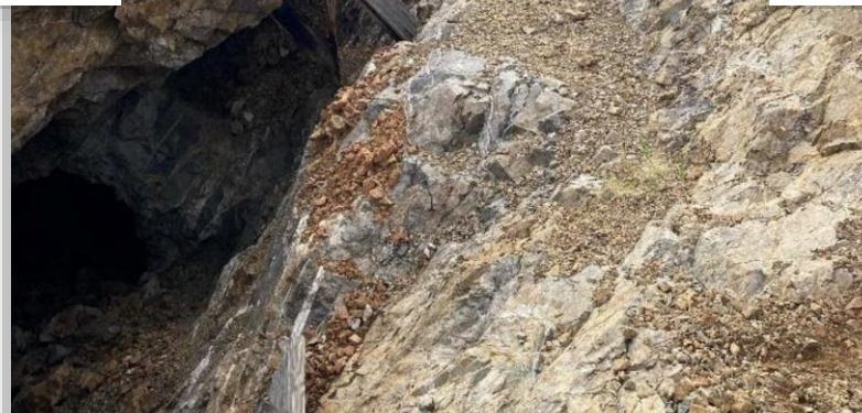
Stope developed on N40W, 50NE zone of sheeted calcite > comb-sucrosic quartz veinlets; Sample No. 101 contained 9.22 ppm Au over 0.5 meters.
