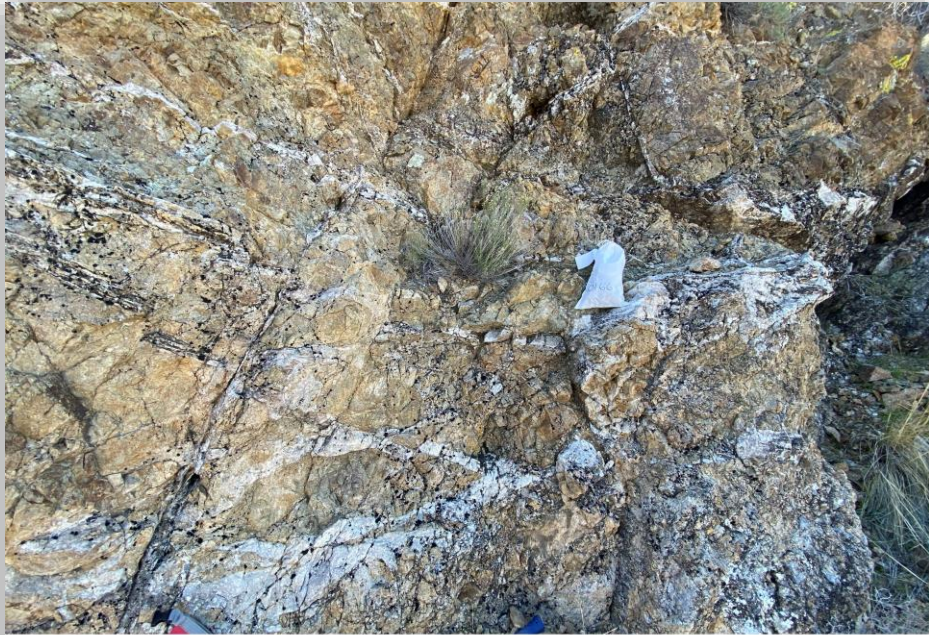
Stockwork chalcidonic quartz veining, Epidote area - Sample # 0166 - 1.5m @ 4.85gpt Au
