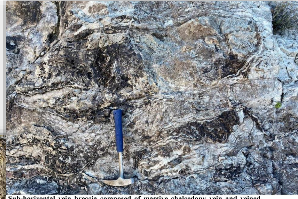
Sub-horizontal vein breccia composed of massive chalcedony vein and veined, silicified fragments cemented by banded, quartz-calcite veins and veinlets. Sample Nos. 0016 & 0017 - 3.0m @ 5.12 g/t Au.
