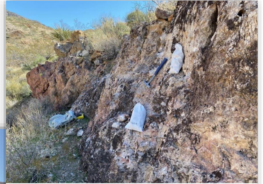
Ledge of quartz-calcite breccia where the Klondyke fault passes beneath a gully to the NE suggesting a highly variable strike and dipping; Sample Nos. 0008 and 0009 contained 2.2 meters @ 3.22 ppm Au.
